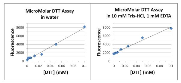
The MicroMolar DTT Assay Kit (catalog number DTT200) includes 5 ml of Dye C55. It is for measurement of 200 samples using 96-well plates. Cuvettes may also be used for measurements.
